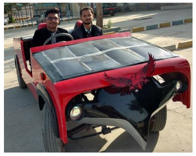
be upgraded up to 50 Km/h by utilizing either a separate gear or pulley mesh. The vehicle is rack and pinion steered. The transmission system is of Drive shaft and engine side and pulley mounted on motor side, the engine contains 5 round gears where as the motor has been equipped with a single pulley only. The batteries get their selves charged when the vehicle runs on engine.
